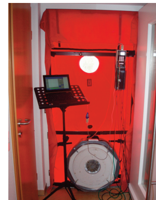
Right: Picture five – Areas of a house being tested for air-tightness
